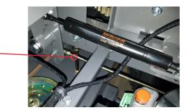
Figure 5.3: Drive Arm Linkage
