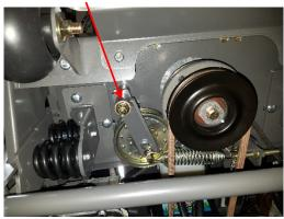
Figure 6.2: Pump Idler Zerk
