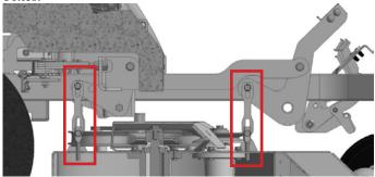
Figure 5.5: Deck Mounting Hardware
