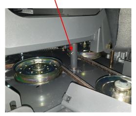
Figure 6.1: Deck Idler Zerk **Pump Idler Zerk**
