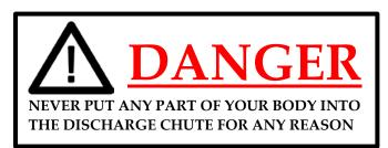
Completely shut down the mower. Use a stick or other long implement to remove any clogged material and then resume normal mowing operations.
