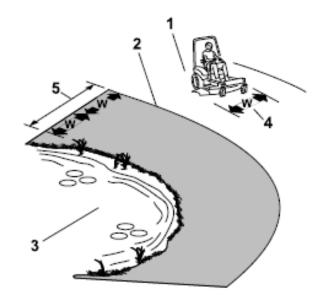
Safe Zone—use the machine here on slopes less than 15° or flat areas.
