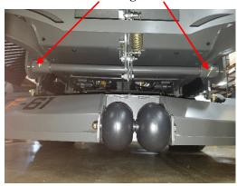
Figure 6.0: Deck Height Zerks
