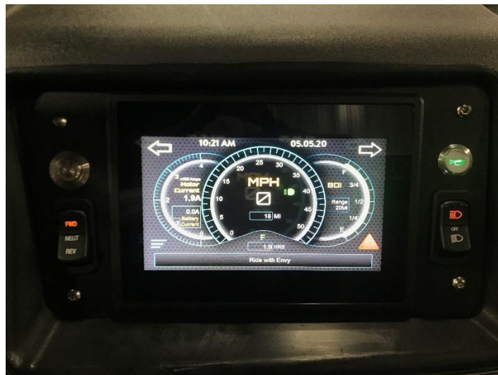
Figure 2: eNVy Control Center
