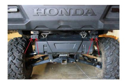
Step 4: Position the mounting brackets on the rear of the machine and loosely mount to the frame using the 4 M10 Hex Bolts and 4 Flat Washers.
