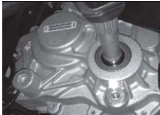
Figure 23: Gearbox Drain Plug
