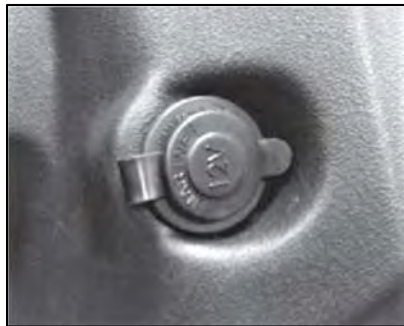
Figure 10: 12V Electrical Outlet
