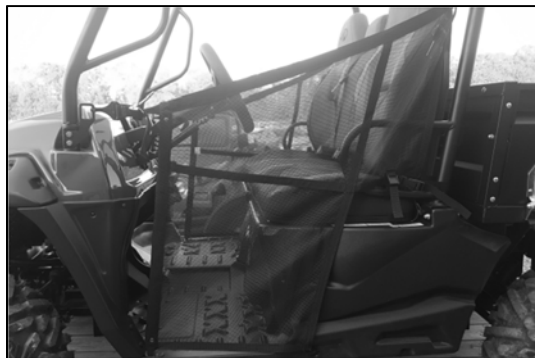
Figure 12: Driver's Side Safety Cab Net
