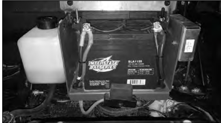
Figure 29: Battery Location Under Hood
