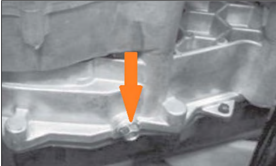
Figure 28: CVT Drain Bolt Location
