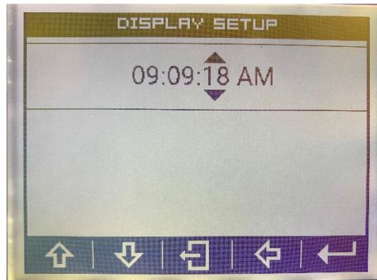
Use the up and down buttons to adjust the seconds. Press the Enter button to move to the minutes. Adjust with the up and down buttons, and then press enter to move to hours. Adjust, and then press enter to confirm the time.
