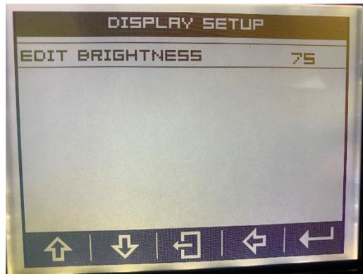
Using the up and down arrow keys will adjust the brightness of the screen from 1 being the lowest and 100 being the brightest.
