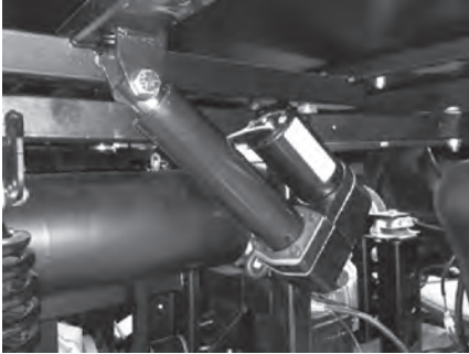
Electric actuator on dump box
