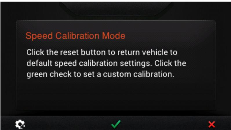
Pressing the reset (first) button will return the display to the default speed calibration settings. Pressing the green checkmark (third) button will begin the process (after verifying this is desired) to set a custom configuration. Instructions will appear to drive exactly one mile and then click Save (green checkmark).
