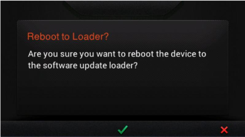
Press the (green checkmark) to reboot to the software update loader. The unit will reboot and display a message to insert a USB drive with the new update files. Follow the prompts on the screen to install the appropriate file.
