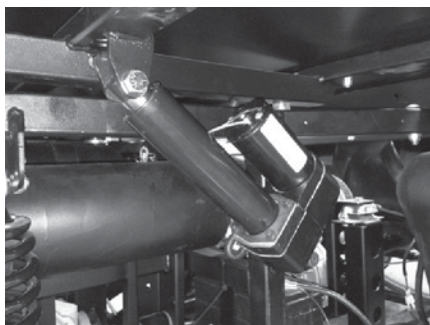
Electric actuator on dump box
