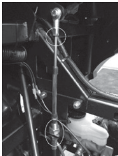
Shift linkage adjustment under hood
