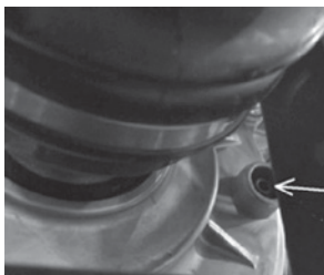
Front Differential Check/Fill plug
