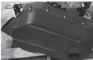
CVT housing shown without vent hoses attached
