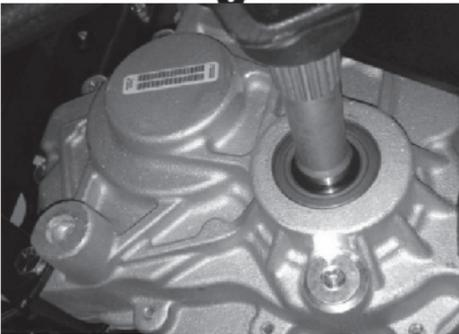
The drain plug is located on the lower front, driver side of the gear case.
