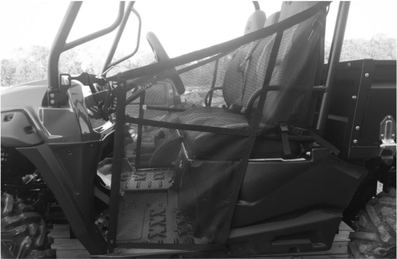
**DANGER:** Falling from a moving vehicle could result in serious injury or death. Always fasten your seatbelt and secure the safety cab net.
