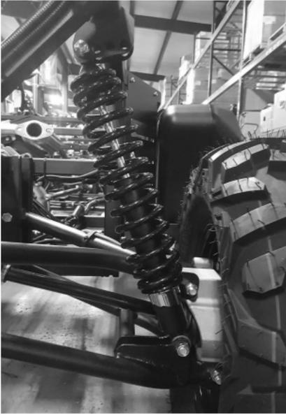
All four shock absorbers have four (4) spring position adjustments, which will tighten or loosen the spring travel rate to adjust the suspension for different terrain and payload conditions. If you plan to haul heavy cargo or have a heavy accessory, like a snow plow, you can tighten the spring rate by moving the silver ring up. In doing so, the vehicle will not squat as much, giving you more ground clearance and better steering control.
