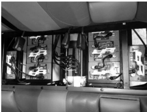
Batteries located under seat
