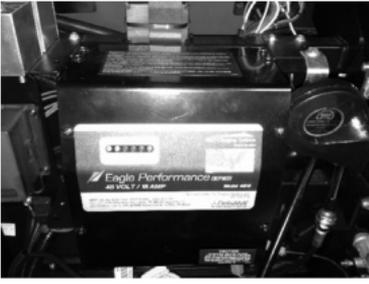
On-board battery charger located under hood
