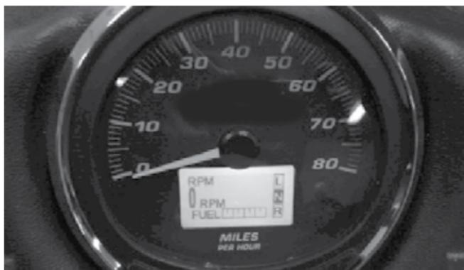
Your Intimidator is equipped with an analog speedometer and a digital LCD screen. High pressure water or soap may damage components. The LCD screen will display the following:
