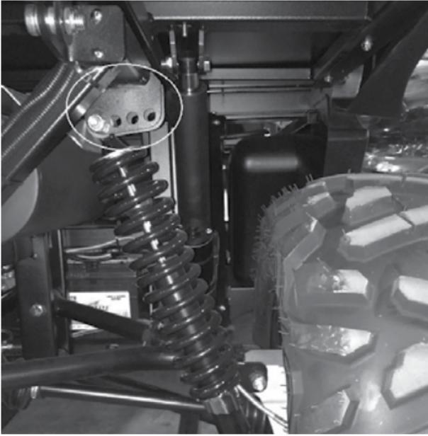
All four shock absorbers have four (4) spring position adjustments on the top, which will tighten or loosen the spring travel rate to adjust the suspension for different terrain and payload conditions. If you plan to haul heavy cargo or have a heavy accessory, like a snow plow, you can tighten the spring rate by moving the silver ring up. In doing so, the vehicle will not squat as much, giving you more ground clearance and better steering control.
