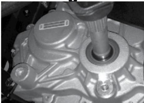
The drain plug is located on the lower front, driver side of the gear case.
