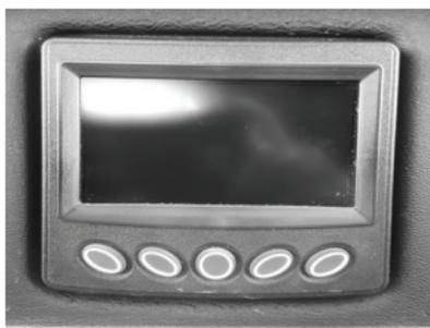
Your Intimidator is equipped with a digital LCD screen, with touchscreen capabilities on the 7" version. General maintenance is not required; however, a soft cloth can be used for cleaning the units. Window cleaner or alcohol can also be used to clean the glass portion of the display. Do not use harsh or abrasive cleaners on the unit.
