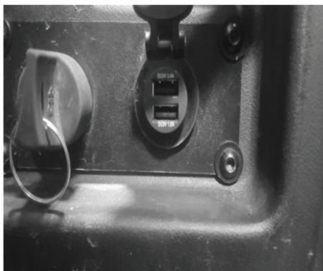
The double USB Port is located on the driver's side next to the ignition switch. **The USB ports are both DC5V but one is 2.4A and the other is 1.0A. They can both be used as chargers for anything that hooks up via USB**
