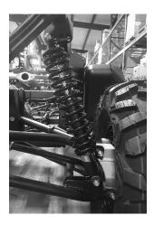
All four shock absorbers have four (4) spring position adjustments, which will tighten or loosen the spring travel rate to adjust the suspension for different terrain and payload conditions. If you plan to haul heavy cargo or have a heavy accessory, like a snow plow, you can tighten the spring rate by moving the silver ring up. In doing so, the vehicle will not squat as much, giving you more ground clearance and better steering control.
