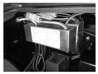
The Intimidator EV has two 48 volt-to-12 volt power converters underneath the hood to run all the 12 volt electronics. Some additional accessories, like lights, can be added. To run large accessories, like a winch, you would need to purchase an Intimidator winch battery kit from Bad Dawg Accessories.
