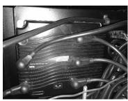
**NOTICE:** The 650amp Curtis controller is water resistant, not waterproof. Avoid spaying the controller with high-pressure water. Do not submerge the controller.
