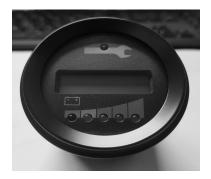
The Battery meter, or BDI, is an auxiliary gauge that displays the percentage of battery life remaining, an hour meter and any error code if one should exist.
