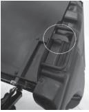
Bed handle and lever to release bed latch
