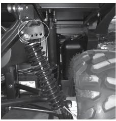
All four shock absorbers have four (4) spring position adjustments on the top, which will tighten or loosen the spring travel rate to adjust the suspension for different terrain and payload conditions. If you plan to haul heavy cargo or have a heavy accessory, like a snow plow, you can tighten the spring rate by moving the silver ring up. In doing so, the vehicle will not squat as much, giving you more ground clearance and better steering control.
