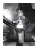
Shift linkage adjustment near gearbox
