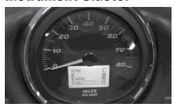
Your Intimidator is equipped with an analog speedometer and a digital LCD screen. High pressure water or soap may damage components. The LCD screen will display the following:
