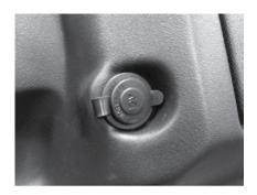
The 12 volt receptacle is located on the passenger side of the dash, left of the glove box.
