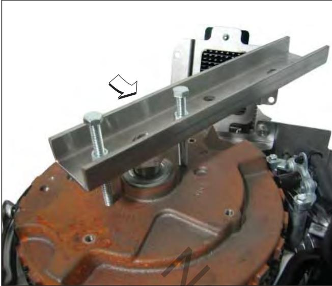
Figure 5-9 Install Flywheel Puller (Part No. 19621).
