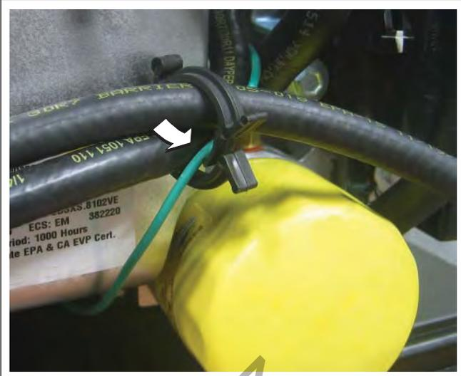
Figure 5-11 Capture Oil Pressure Switch Wire in Clip.
