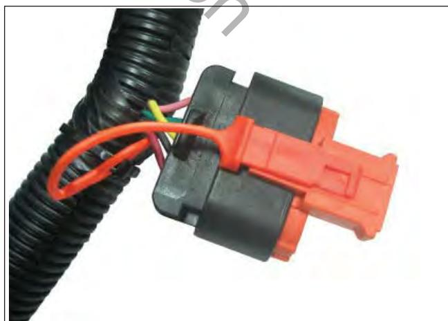
Figure 1-2 Data Link Connector (DLC).
