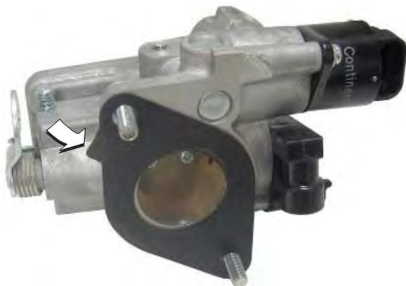
Figure 5-21 Throttle Body Gasket.
