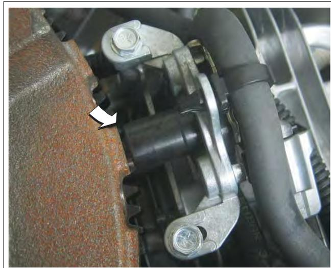
Figure 5-8 Adjust CKP Sensor Gap.
