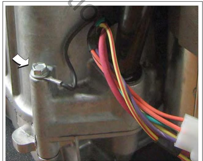
Figure 5-12 Fasten Ground Wire Ring Terminal to Boss.
