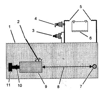
Use the example above. The current flow from the welder to the ground clamp of the welder will not damage any associated components.
