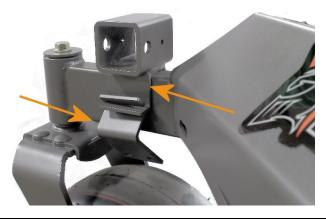
• Set in place the Two Part Receiver Clamp as shown.
