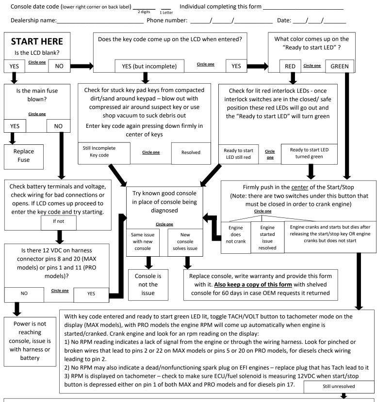
Check with Known good console, if engine cranks but still does not start the issue is outside the console. If engine starts then Replace console, write warranty and provide this form with it. Also keep a copy of this form with shelved console for 60 days in case OEM requests it returned
