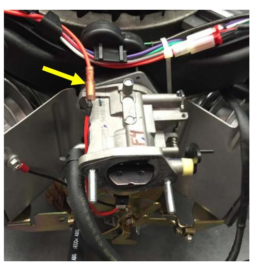
3. Remove the air cleaner base and disconnect the carburetor solenoid power wire indicated by the yellow arrow
