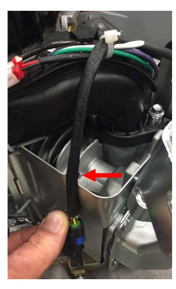
7. Assure that the E-Choke wiring exits across the baffle in the location indicated by the red arrow below. Then, install the provided carburetor gasket and reinstall the air cleaner base. Torque the air cleaner base nuts to 60 in-lbf
