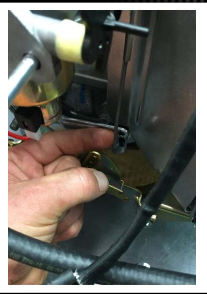
4. Remove the throttle linkage from the governor lever
