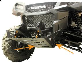
• Using the factory bolts (previously moved from the indicated location), secure the skid plate to the frame.
