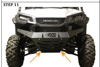
• Tighten the Factory Bolts at the bottom of the skid plate.
