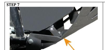
• Secure the Plastic Mounting Bracket using the provided ¼-20 x 1" Button Head Bolt with flat washer and Nylock Nut.
