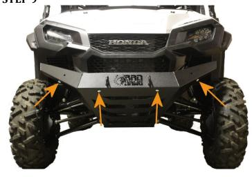
• Begin the tightening sequence by first tightening the four front bolts indicated here.
