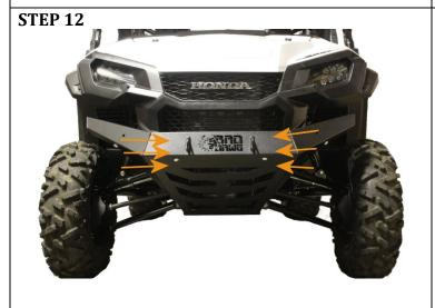
• Tighten the six inside bolts of the Side Mounting Brackets.
