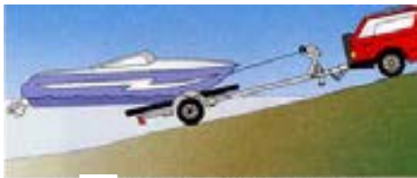
Fig 10 Launching from a Bunk Trailer on an average grade ramp
