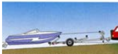
Fig 9 Launching from a Roller Trailer on a shallow ramp
