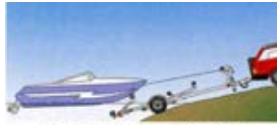
Fig 7 Launching from a Roller Trailer on a steep ramp
