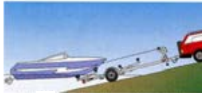
Fig 8 Launching from a Roller Trailer on an average grade ramp
