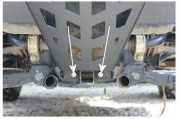
1. Using the provided 3/8" x 1" Hex Head Bolts, loosely bolt the Skid Plate Support (item 4) to the bottom of the frame as shown.
